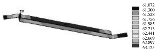
图 4 额定工况时线圈温度分布 Fig.4 Temperature of windings at rated load
